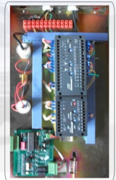
Mobular control panel with loop detector and RS 485 Card (Inbuilt)
